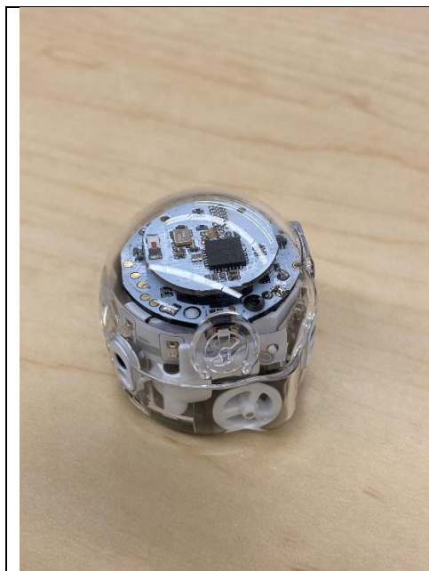
Photo 1: Press power button at top of Evo – the robot it will light up.
